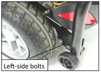
Figure 1: Rear Bumper Installed
